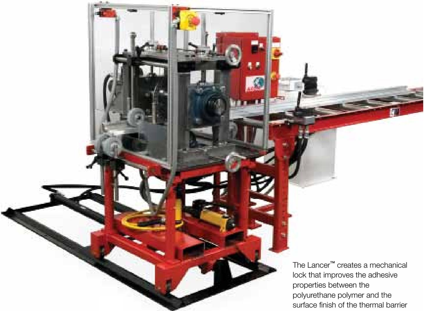
The Lancer™ creates a mechanical lock that improves the adhesive properties between the polyurethane polymer and the surface finish of the thermal barrier pocket as used in an aluminum window, door or curtain wall profile.
