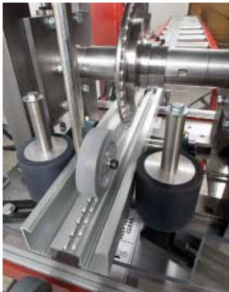
The lancing wheel travels along the lugs to produce lanced indentations that bend down into an extrusion cavity
