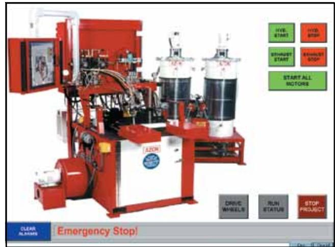
All motors start and stop from the main screen including the hydraulic power unit, fume extractor and chemical agitators.
