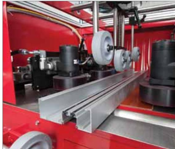
A dual cavity with MLP™ (mechanical lock profile) is debridged to eliminate the metal-to-metal contact resulting in a structural composite of aluminum and polymer to create the strongest thermal barrier for aluminum extrusions.
